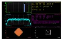
Margin testing requires more than ideal signals. Impairments, noise and interfering signals must be added in order to obtain the required results. MODULAR, with its built-in impairment tool, featuring carrier feed-through and quadrature error and imbalance and multi-carrier capability, makes it possible to do all this with just a single unit.
