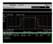
High quality signals with multiple channels/carriers require an additional feature - uncorrelated payloads. MODULAR allows complete definition of pseudo-random binary sequences (PRBS) for payloads, controlling both the generation polynomial and the seed values in a carrier-by-carrier basis. Additionally, carrier phase can be defined by the user or at random. This feature sharply reduces the PAPR (Peak to Average Power Ratio), hence improving linearity, dynamic range and SNR.
